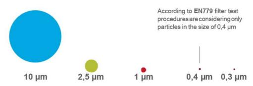
According to ISO 16890 filter test procedures are considering the range from 10 µm-0,3 µm
